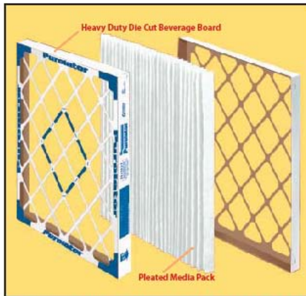
Two mating pieces of die cut beverage board form a double wall frame around all four edges of the filter. Hi-E 40 filters will not rack or warp under normal operating conditions.
